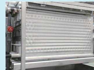
ThermoJinn water chiller Plate type evaporator uses high quality stainless steel (SUS304&SUS316) plate, special welding process. The cooling capacity channel inside the evaporator is smooth and the surface is smooth. Suitable for working conditions with large flow and low outlet water temperature.
